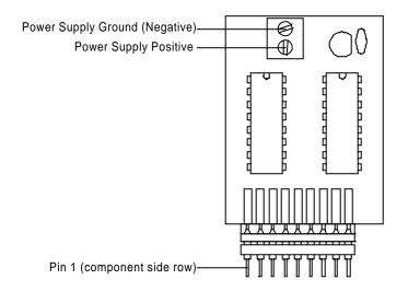
The OBM-1 requires a DC supply in the range 8 to 35 Volts between its 'Power Supply Positive' and 'Power Supply Ground' terminals to power its on-board circuitry. This supply must share the same ground potential as the MTP circuit on which it is fitted. This supply must be adequately smoothed to maintain a minimum voltage of 8V at all times. In most cases, the same supply which powers the MTP circuit logic can be used to also power one or more OBM-1 circuits.
