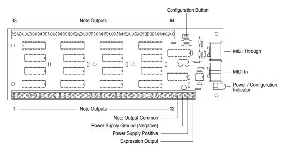
There is one screw terminal connection for each note output. One lead of each output device is connected to the appropriate output terminal of the MTP-8. The other leads of all the output devices must be connected together and this common point connected to the 'Note Output Common' terminal. If the polarity of the output devices is important, connect the positive lead of the output device to the common terminal.
