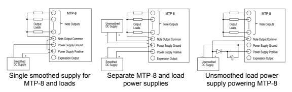
A simple unsmoothed DC power supply can be constructed from a low-voltage mains transformer and full-wave bridge rectifier. If a diode and capacitor is used to provide smoothed power to the MTP-8 as in the example above, the capacitor must be sized such that the ripple voltage does not cause the supply to drop below 8 V.
