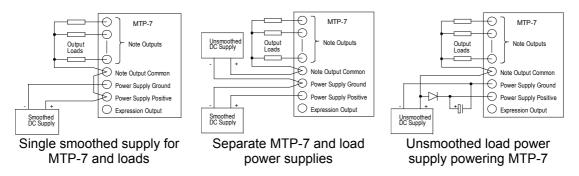
A simple unsmoothed DC power supply can be constructed from a low-voltage mains transformer and full-wave bridge rectifier. If a diode and capacitor is used to provide smoothed power to the MTP-7 as in the example above, the capacitor must be sized such that the ripple voltage does not cause the supply to drop below 8 V.
