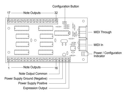
There is one screw terminal connection for each note output. One lead of each output device is connected to the appropriate output terminal of the MTP-7. The other leads of all the output devices must be connected together and this common point connected to the 'Note Output Common' terminal. If the polarity of the output devices is important, connect the positive lead of the output device to the common terminal.
