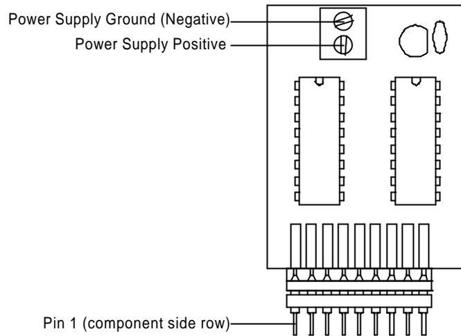
The OBM-1 requires a DC supply in the range 8 to 35 Volts between its 'Power Supply Positive' and 'Power Supply Ground' terminals to power its on-board circuitry. This supply must share the same ground potential as the MTP circuit on which it is fitted. This supply must be adequately smoothed to maintain a minimum voltage of 8V at all times. In most cases, the same supply which powers the MTP circuit logic can be used to also power one or more OBM-1 circuits.
